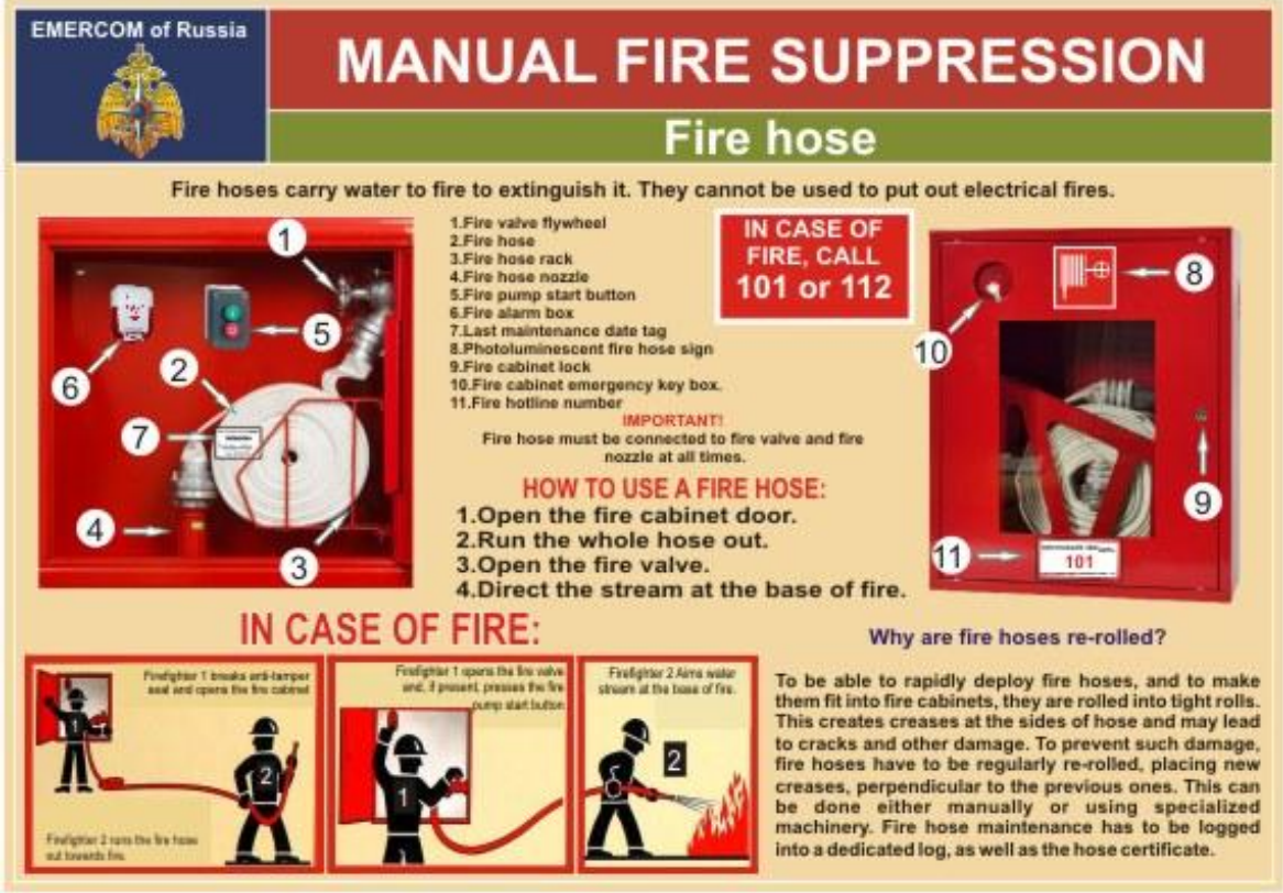
Figure 21 — Internal fire hydrant
