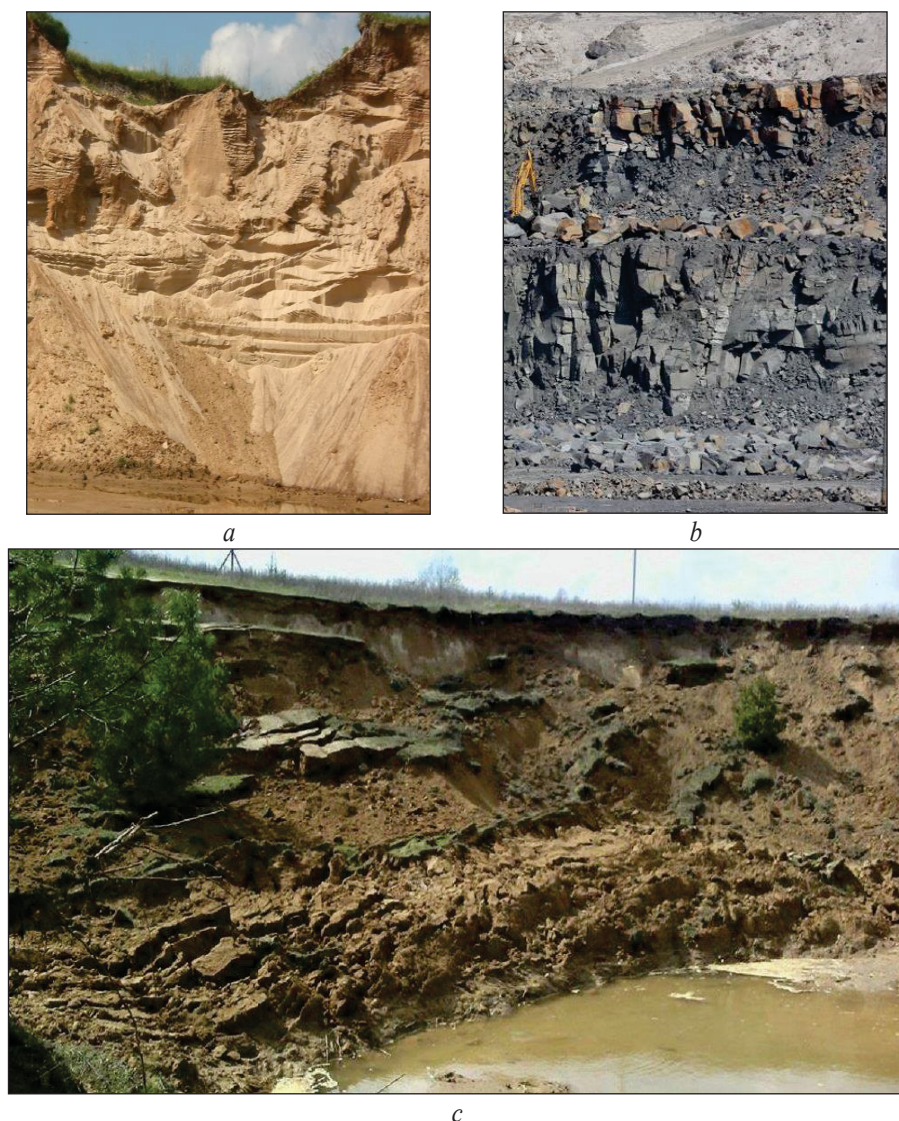
Fig. 4. Gravitational processes in the sides of the quarries: a) talus in the Leskovichi quarry for sand extraction (Shumilinsky district, 2008); b) talus in the Mikashevichi quarry for the extraction of granite (Luninetsky district, 2010); c) landslide in the open pit «Khmelevskie prudy» for sand extraction (Minsk district, 2015) [10]
